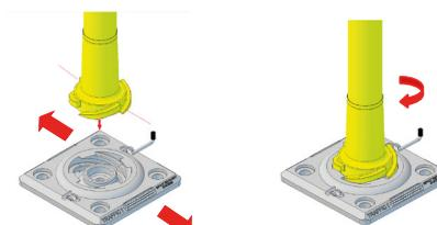
1. Insert the threaded post into base with holes aligned 90° to keeper pin slot.
